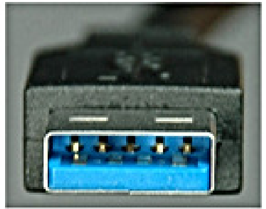
USB 3.0 A plug pinout
