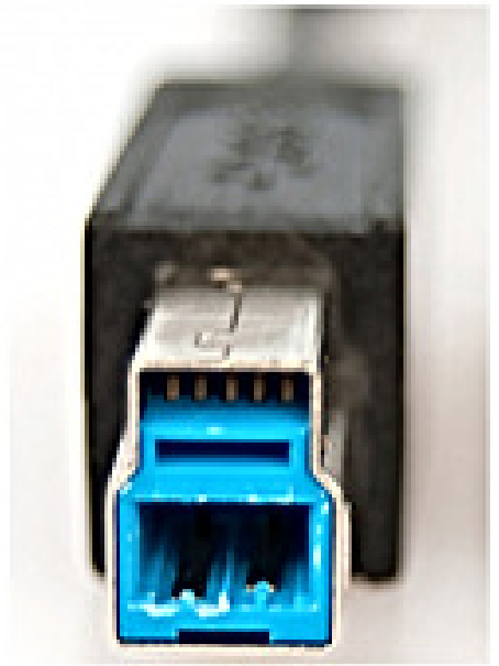
USB 3.0 B plug pinout
