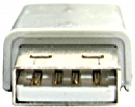
USB 2.0 A plug pinout
