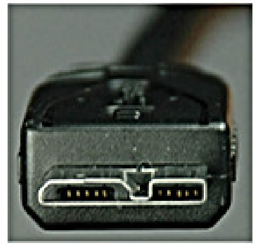
USB 3.0 micro-B plug pinout
